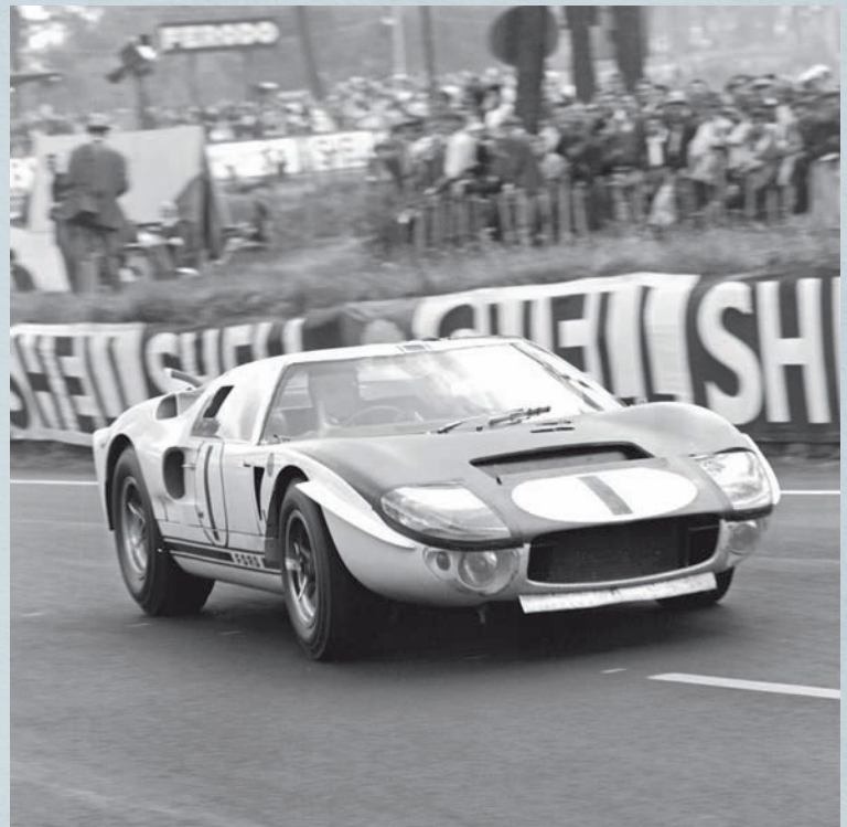
The car raced by McLaren and Miles at Le Mans in 1965, GT/106, came out of Slough as a plain-Jane Ford GT. When it was fitted with a 427, it became a Mark II. Had it subsequently been retrofitted with a 289, it would have been renamed a Mark I. Confused yet?
